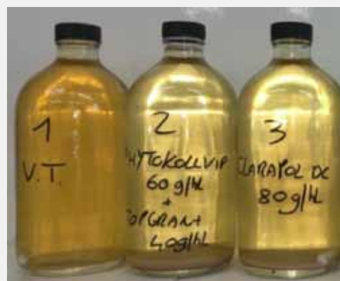
Colour browning in control wine and in treated wine. Oxidation test with H_2O_2
